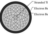
Stranded Tinned Copper Conductor Electron Beam Cross-linked Insulation Electron Beam Cross-linked Sheath
